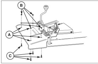
Figure 6. Install Deflector A. 13/64 Hole Locations B. Nylock Nuts
